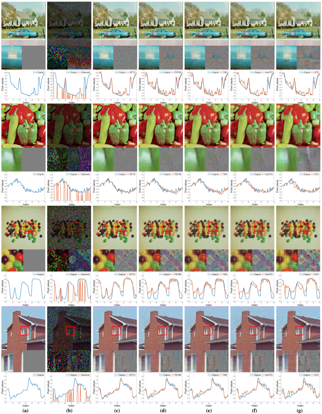
FIGURE 6 Examples of color image inpainting with SR = 30\% . From top to bottom are respectively corresponding to “House,” “Peppers,” “Beans,” and “Wall.” (a) Original; (b) Observed; (c) WTTC; (d) PSTNN; (e) TNN; (f) HaLRTC; (g) NTD
